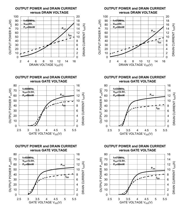
RoHS Compliance , 400-470MHz 30W 12.5V, 3 Stage Amp. For MOBILE RADIO
