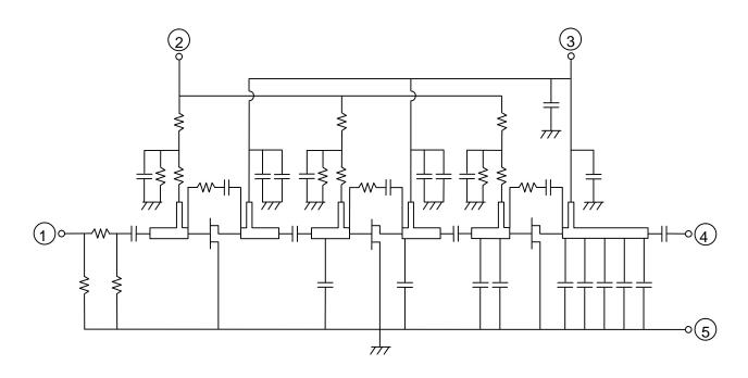
RoHS Compliance , 400-470MHz 30W 12.5V, 3 Stage Amp. For MOBILE RADIO
