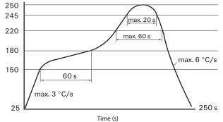
Resistance to soldering heat - Reflow profile
