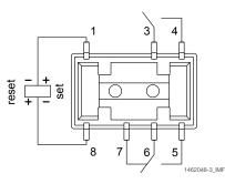
Contacts are shown in reset condition. Contact position might change during transportation and must be reset before soldering.
