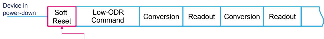
Figure 8. Low-ODR mode enable sequence
