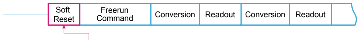
Figure 7. Freerun mode enable sequence
